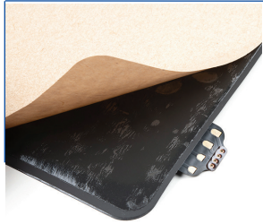
Example of an LEL component with a flex PCB termination and pressure sensitive adhesive film applied for integration
